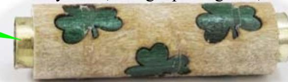
onto the barrel using 2 part epoxy. Secure with a small bar clamp to ensure a tight joint. Once the epoxy has cured, sand the ends flush to the brass tube again and return to the lathe for final turning and finishing using the finish of your choice.
